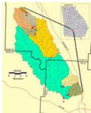
Figure 1. The Little River Watershed is 334 km 2 (30-40% agricultural). All analysis was done on sub-basin K, a 16.8 km 2 area in the north, with the most nutrient data available of any of the basins. The Southeast Watershed Research Lab has collected hydraulic, nutrient and climatic data continuously since 1965.
